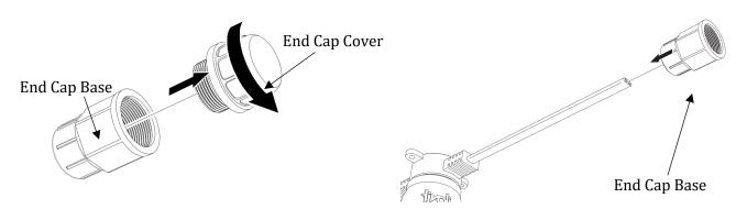
6. Attach the end cap cover onto the end cap base and tighten.
