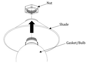
8. Attach the globe or the shade assembly to the socket.
